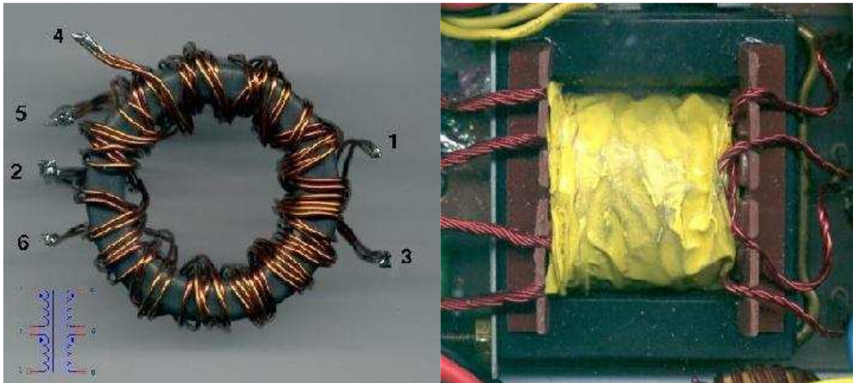
Left - Home Made Transformer. Commercial Transformer - Right
