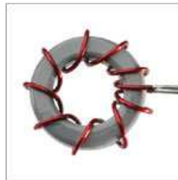
Toroid from ITL 100 inductor (Wilco Corp). (Remove the thick wire before winding! :-)
