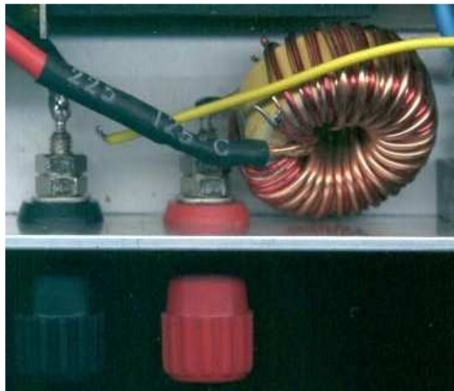
My system's input choke, obtained from an old PC power supply.
