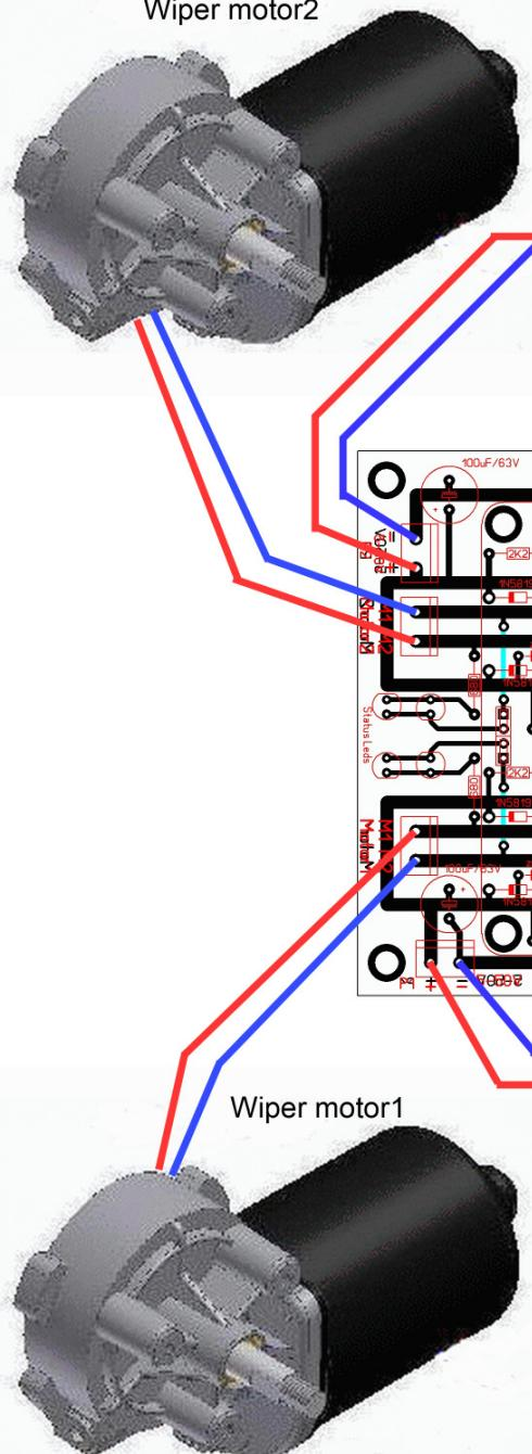
Connection Diagram of the AMC1.5 and DSMhb1.2b with two wiper motors and two potentiometers
