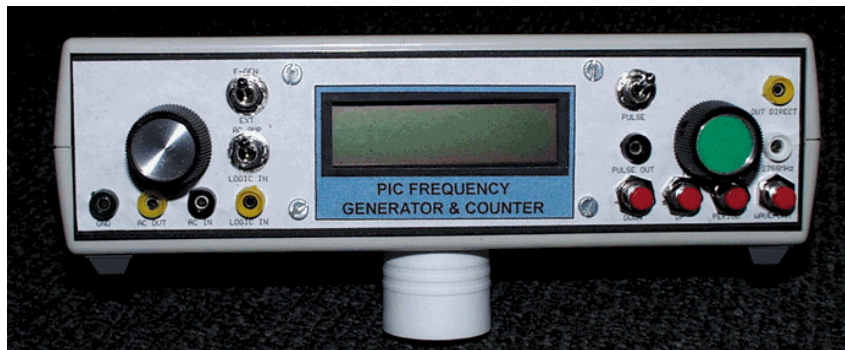
PIC-Gen front panel. The waveform button is bottom far right. The switch marked "pulse" (top right) is the on/off switch in the final model.
